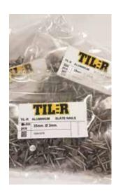
Another example of TIL-R helping contractors is their copper and aluminium nails for slate. These have been designed to meet all the requirements of BS 5534, which stipulates a minimum gauge of 3mm, a head size of 10mm minimum and a penetration into the batten of a minimum 20 to 22mm. TIL-R's nails provide good penetration into batten without damage, and with a
