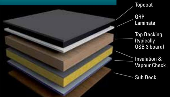
This diagram demonstrates a typical warm roof construction and can be used as a guide, however we do recommend that you check current building regulations before commencing work. Warm roof constructions generally require edge trims with a greater drop, such as the A250 and B300, due to the additional thickness of the roof.
